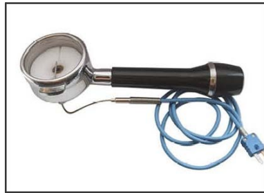
A-MC-1046A PORTAFILTER WHIT THERMOCOUPLE
